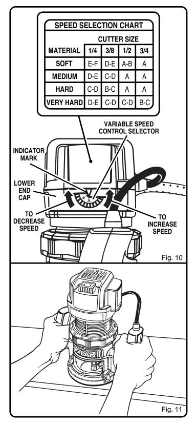
The best rate of feed is one that does not slow down the router motor more than one-third of its no-load speed. If the router is fed too fast, it will take large chips out of the wood and leave gouge marks. If the router is fed too slow, it will scorch or burn the wood.
